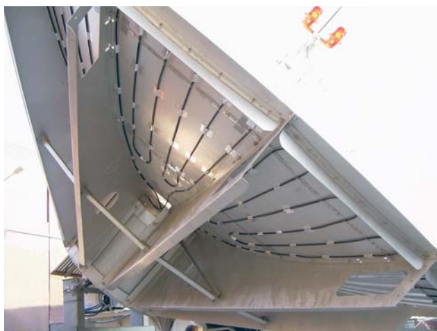
Satellite dish protection against snow and ice
