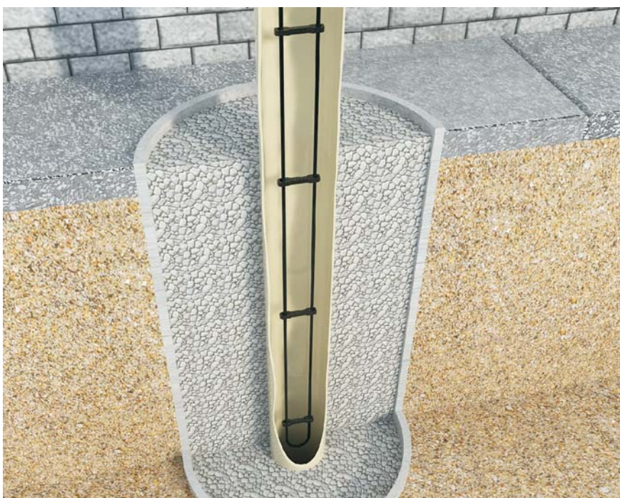
Heating cable installation below the ground surface
