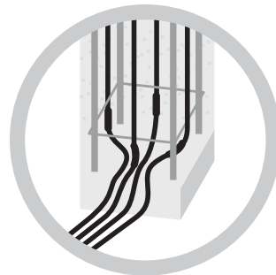
Installing heating cables in a concrete pillar
