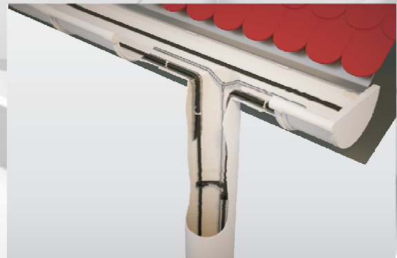
Installation in the transition spot between the gutter and the downpipe
